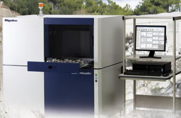
The need for quick determination of elements in geological samples has been increasing. Semi-quantitative analysis, with modern XRF instruments, may be performed without any reference materials. SQX is Rigaku's semi-quantitative analysis (standardless analysis) program to obtain concentrations by theoretical calculation using the fundamental parameter (FP) method.
