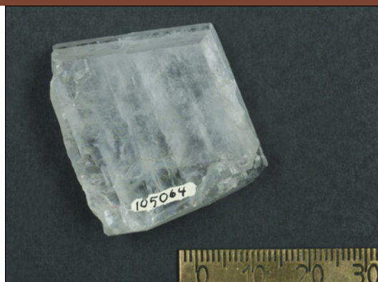
Dolomite sample MGM#105064 from the Harvard mineral collection. This material—already characterized for major element contents—is now available through IAGeo.com and is also under further investigation as a possible isotope reference material.
