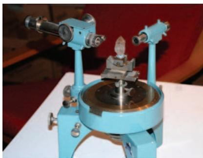
**FIGURE 1** A Unicam single-circle optical goniometer, like the one described in the text. The quartz crystal here is much larger than those I used for teaching.
