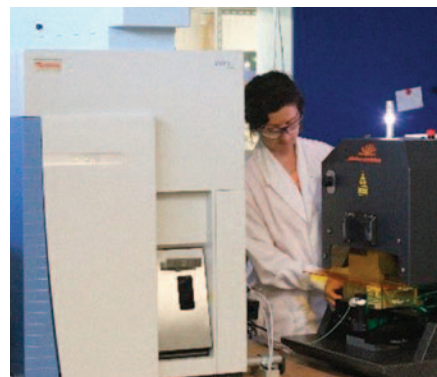
FIGURE 2 Swiss mass spectrometer manufacturer TOFWERK's icpTOF system being used in conjunction with a Photon-Machines laser ablation system. The vertical mount geometry has the advantage of reducing the amount of floor space needed for the instrument. The horizontally oriented time-of-flight segment is visible at the top of the instrument. PHOTO: M. CUBISON (2016).
