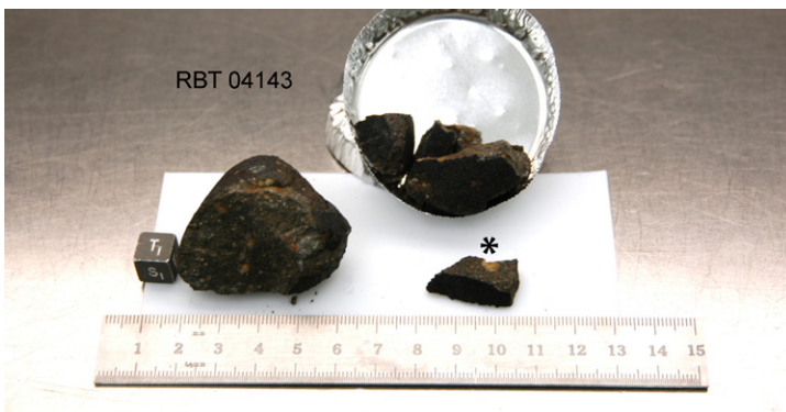
FIGURE 1 NASA image of the Robert Massif (RBT) 04143 carbonaceous chondrite (CV3) found in Antarctica by the U.S. Antarctic Search for Meteorites (ANSMET) program. The cube pictured is 1 cm along each edge and the ruler is in cm. The light-colored object in the piece below the * is an impact melt pocket that formed by in situ melting of this carbonaceous chondrite.
