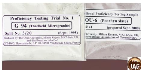
**FIGURE 1** Sample sachets from earlier rounds of the IAG's GeoPT proficiency testing programme. Each unit contains around 50 g of whole-rock powder.
