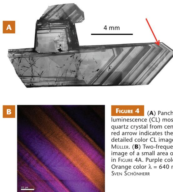
**FIGURE 4** (A) Panchromatic cathodoluminescence (CL) mosaic of a large quartz crystal from central Norway. The red arrow indicates the location for the detailed color CL image. IMAGE CREDIT: A. MÜLLER. (B) Two-frequency, false color CL image of a small area of the quartz crystal in FIGURE 4A. Purple color  $\lambda = 411\ \text{nm}$ ; Orange color  $\lambda = 640\ \text{nm}$ . IMAGE CREDIT: SVEN SCHÖNHERR
