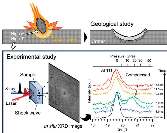
**FIGURE 1** Schematic illustration of the new experimental shock system set up at the Photon Factory Advanced Ring (Japan) and, at right, some resultant sample data. The time-resolved X-ray diffraction data shows the dynamics of the Al (111) plane from shock compression to release (following the time arrow).
