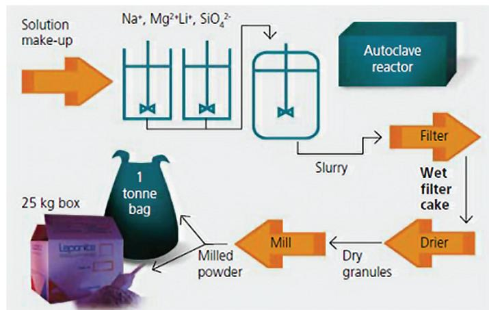
**FIGURE 2** Schematic flowchart depicting the general process for making Laponite®. BYK Additives and Instruments
