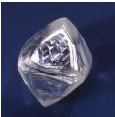
Rounded diamond octahedron showing etch "trigons." 5.26 cts (8 mm across), Kimberley, South Africa. AMNH 91708
