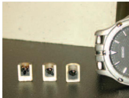
Polycrystalline zircon capsules containing quenched basaltic melt
