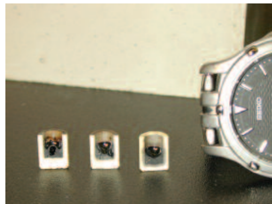
Polycrystalline zircon capsules containing quenched basaltic melt
