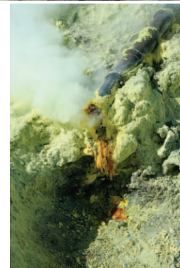
Ceramic pipes used to channel and condense sulfur gas into molten sulfur
