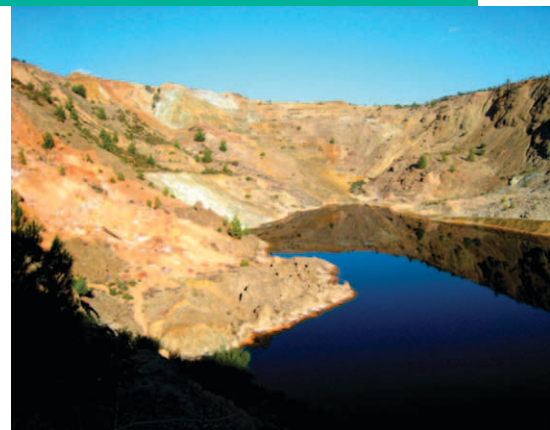
Acid sulphate waters in the abandoned Limni Mine, a Cyprus-style Cu deposit
