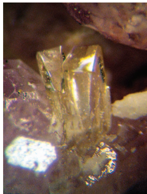
FIGURE 2 \text{K}_3\text{Ti}^{4+}\text{Fe}^{3+}(\text{SO}_4)_4\text{O} \cdot 2\text{H}_2\text{O} crystals (about 1.5 mm tall) on coquimbite, \text{Fe}_2(\text{SO}_4)_3 \cdot 9\text{H}_2\text{O} . PHOTO AND SPECIMEN: A. KAMPF
