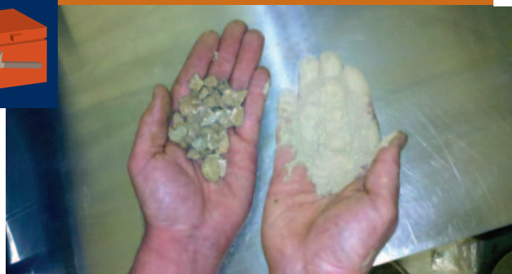
FIGURE 3 An example of a phosphate starting material and end product from the Aerodynamic Impact Reactor
