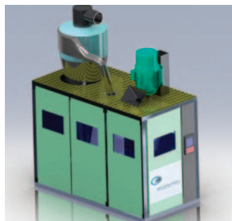
FIGURE 1 Model of the Aerodynamic Impact Reactor (patent pending). The reactor's height is approximately 2 metres.
