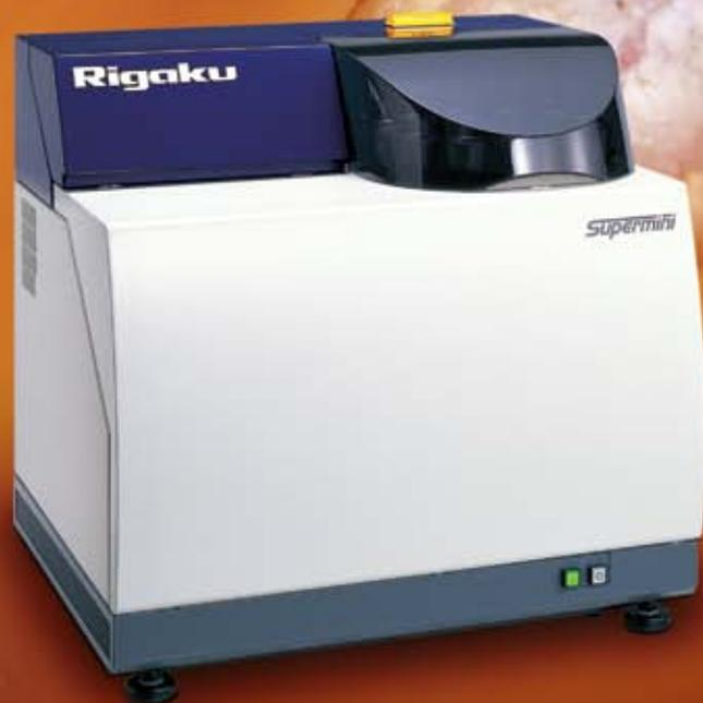
The Supermini is a WDXRF spectrometer delivering exceptional resolution and low limits of detection.
