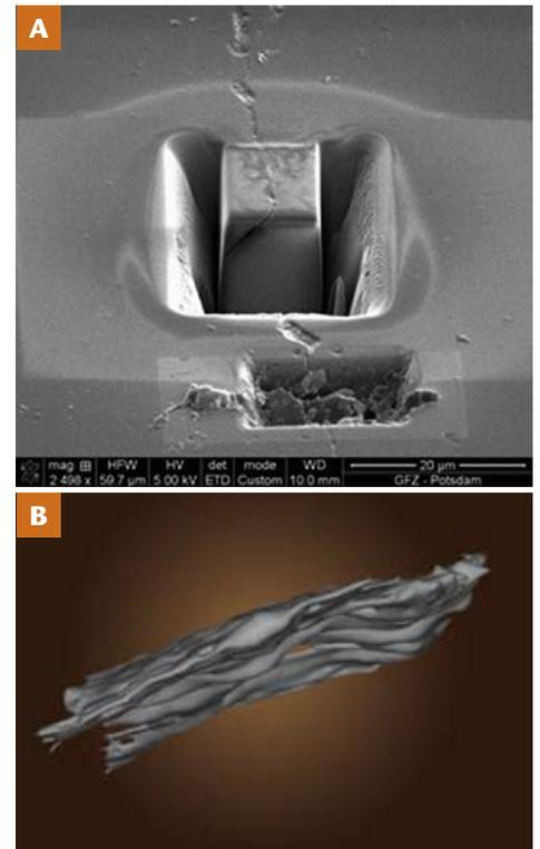
**FIGURE 3** (A) 10 μm cube milled into the sample surface as it appeared prior to 3-D imaging. The trace of the grain boundary across the top and front faces of the cube is clearly visible. (B) Two-dimensional projection of the 3-D geometry of a grain boundary between two quartz crystals. The smallest visible topographic features are of the order of a few tens of nanometers in size.
