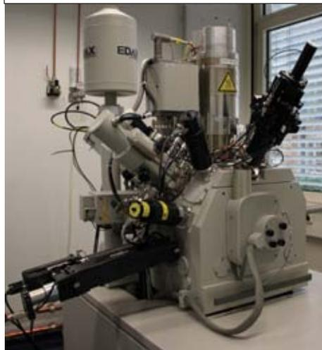
**FIGURE 2** Photo of the Potsdam FEI Quanta dual-beam tool, which in many ways has the appearance of a scanning electron microscope. Above: cartoon showing the general layout of the sample and the two probe beams. COURTESY OF FEI COMPANY
