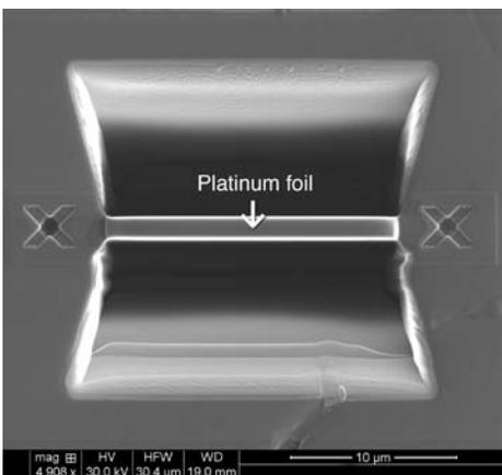
**FIGURE 1** Image of an ~800 nm thick foil milled from a sample. The foil includes a thin layer of platinum metal, which was deposited above the film in order to protect the underlying material. Such “single-beam” applications have been available to the mineralogist for nearly a decade.
