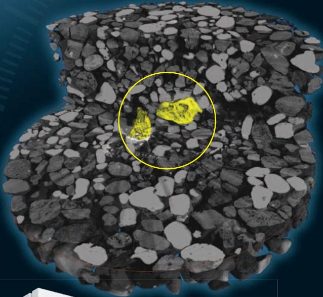
Micro-CT non-destructively reveals density differences in a wide range of rock or soil samples. The exact 3D location, volume and surface of particles or the permeability of the entire sample can be determined.
