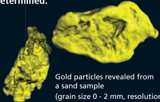
Gold particles revealed from a sand sample (grain size 0 - 2 mm, resolution 10 µm)
