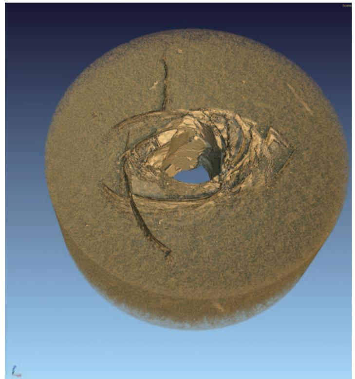
**FIGURE 2** An example of a micro-CT image from a simulated bore hole breakout in shale. The outer diameter of the sample is 20 mm, and the fracture width is of the order of 50  $\mu\text{m}$ . IMAGE COURTESY OF THE HELMHOLTZ ZENTRUM POTSDAM
