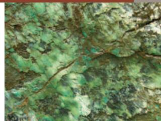
Ni serpentine of New Caledonia. Nickel deposits in New Caledonia form by intense weathering of serpentinites under tropical conditions.
