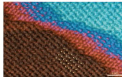
Atomic-scale imaging reveals the mechanisms of crystal dissolution and growth. The image illustrates atomic-scale resolution of a calcite surface showing protruding oxygen atoms of the CaCO<sub>3</sub> structure on a {1014} surface; discrete atomic structure is revealed at the dissolving crystal front. Dissolution details were imaged by atomic force microscopy (AFM dimension fastscan, Bruker Nano Surfaces operating in peak force tapping mode).
