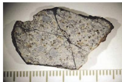
**FIGURE 3** Slice of one of the Chelyabinsk meteorite stones showing chondrules and melt-filled veins. PHOTO CREDIT: LABORATORY OF METEORITICS, VERNADSKY INSTITUTE, RUSSIA
