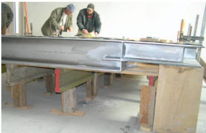
**FIGURE 3** A view of the stainless steel frame used to support the machine 70 cm above the concrete floor
