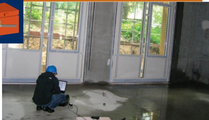
**FIGURE 1** An engineer from Paris measures the magnetic field stability and mechanical vibrations in the second proposed location for the new facility.
