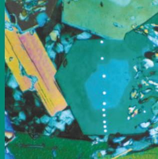
Thin section photomicrograph (crossed-polarizers) of zoned hexagonal tourmaline (grain diameter ~0.4 μm) with chlorite (dark blue), phengite (orange and pink), and epidote (inclusions in tourmaline). The measurement spots produced by SIMS are visible as white dots.
