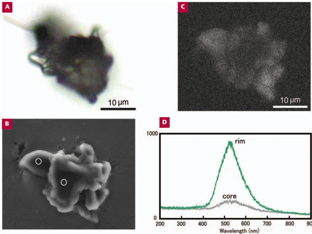
**FIGURE 5** Images and cathodoluminescence (CL) spectra of an S-type microdiamond in dolomite marble (after Yoshioka and Ogasawara in press). **A:** Photomicrograph of analyzed grain. **B:** Secondary electron SEM image of analyzed grain. Small circles are locations from which CL spectra were obtained. **C:** CL image at the peak wavelength (523 nm) of the strongest CL band. **D:** CL spectra of core and rim.
