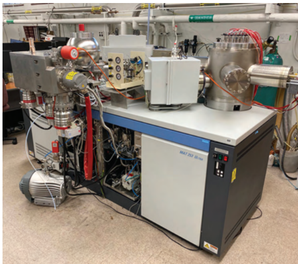
FIGURE 3 Continued use of advanced analytical equipment has been a key factor in the development of organic geochemistry. Shown here is the prototype MAT 253 Ultra mass spectrometer used for clumped isotopologue measurements in Dr. John Eiler's laboratory. PHOTO COURTESY OF DR. ALEX SESSIONS OF CALTECH, USA.
