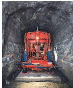
The prototype Cannister Hole Boring Machine "Sanna", developed by Posiva, Finland. Source: Posiva Oy
