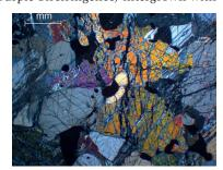
A feldspathic harzburgite from the northern limb of the Bushveld Complex, South Africa, showing coarse-grained amoeboidal olivine, intimately intergrown with surrounding cumulus-textured primocryst enstatite, showing fine lamellar exsolution of calcic pyroxene, and interstitial plagioclase feldspar. The opaque grains intergrown with the olivine or as subhedra adjacent to it are chromites. Photo courtesy of Siyasanga
