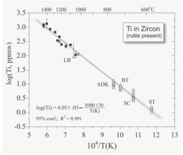
The Ti-in-zircon thermometer was calibrated experimentally by Watson and Harrison between 1025 and 1450°C and by analysis of natural zircons known to have crystallized at 580 to 1070°C on the basis of independent geothermometers. Ti, a tetravalent ion under all relevant
