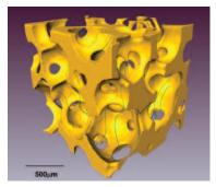
X-ray microtomography image of a bioactive calcium silicate glass scaffold, with calculated fluid flow lines, used as a bone-regenerative scaffold for regions with low tensile loading, e.g. in facial or spinal applications. COURTESY OF GOWSIHAN POOLOGASUNDARAMPILLAI, IMPERIAL COLLEGE
