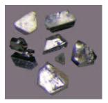
Optical image of synthetic crystals of platinum-rhodium alloy grown by high-temperature vapor deposition (bottom-centre crystal is ~1 mm in diameter). PHOTO COURTESY JAMES M. BRENAN
