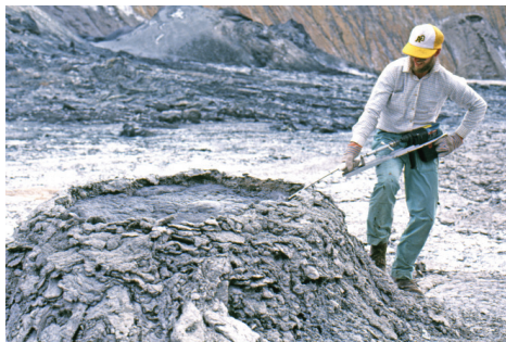
Figure 3 – Harry Pinkerton with a vane viscometer, measuring the viscosity of natrocarbonatite in a miniature hornito, September 1988
